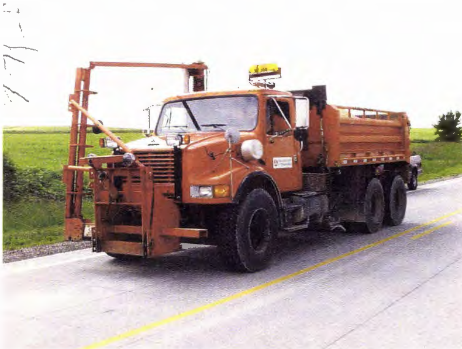
Figure 4-4 Test Truck Provided by IDOT for Strain Data Collection
