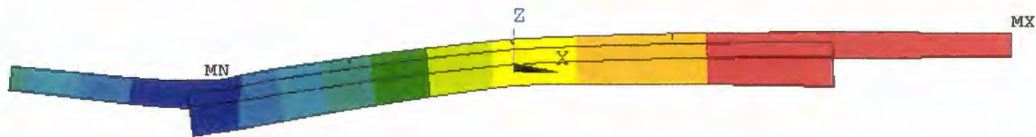
Figure 4-7 Example of Composite Pavement Deflected Shape (9-kip Load) (Cross-Section View – Exaggerated Scale)
